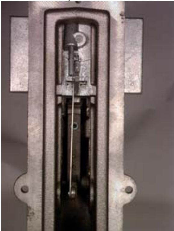
6. Remove the four  $\frac{1}{4}$  - 20 socket head cap screws from the table slide assembly. They are located at bottom mid-section of table slide, and hold the table slide assembly to the machine casting.
