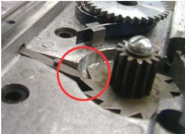
Move the handle to the 9 O'clock position. If the machine is adjusted properly, the top of the pawl should be flush with the top of the flat gear on the escapement wheel assembly. You should be able to run a fingernail across the flat starburst gear and across the pawl assembly.
