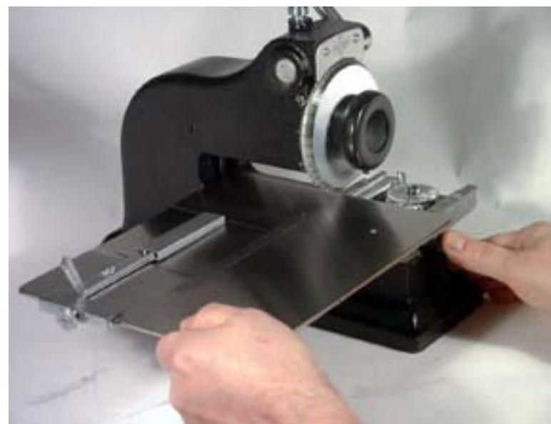
4. While holding the table with your left hand, push in and hold the space button (2-24) and slide the table off the machine to the left.
