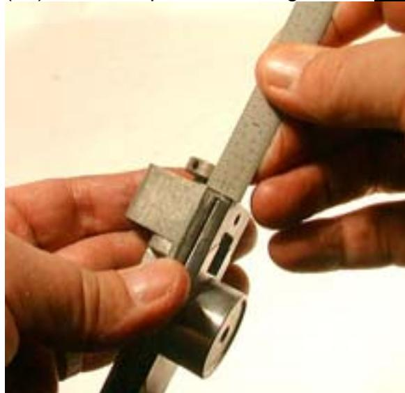
2. Slide the new ram from the bottom up through the dove-tail section of the casting, then replace plunger spring (46) into hole at top of casting and screw the depth adjustment screw into the ram until the operating handle can be pulled down no further than the 9 o'clock (horizontal) position.
