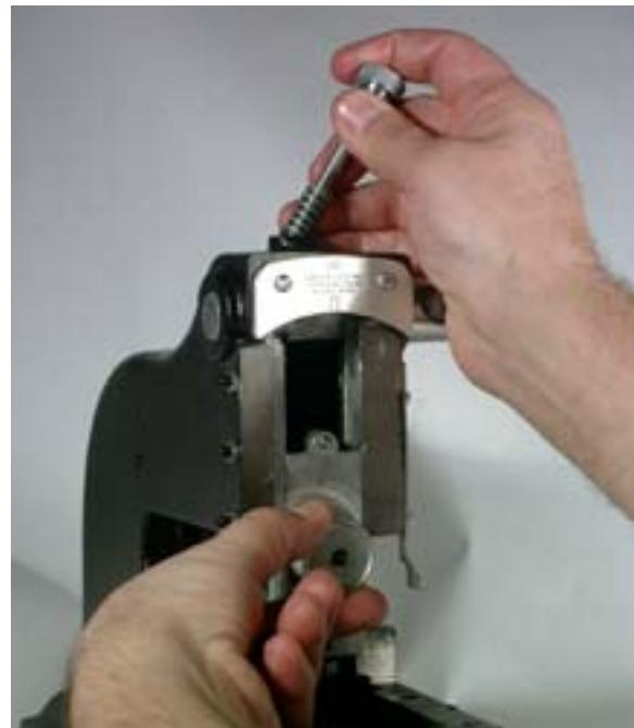
8. Unscrew the depth adjustment screw (39-44) from the ram. The ram can then be pushed down and off the machine.
