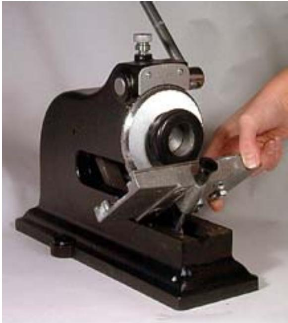
7. Lift the table slide assembly from the machine base and remove.
